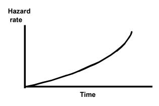
Increasing hazard rate. Scheduled replacement of a part will reduce the probability of failures.
