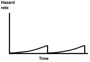
Increasing hazard rate with near failure free life. Scheduled maintenance will ensure near failure free probability.
